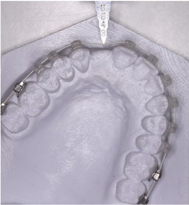
Figure 1 Demonstration of the indenter positioned in the middle of the unsupported wire between maxillary central incisor and canine during the experiment.
